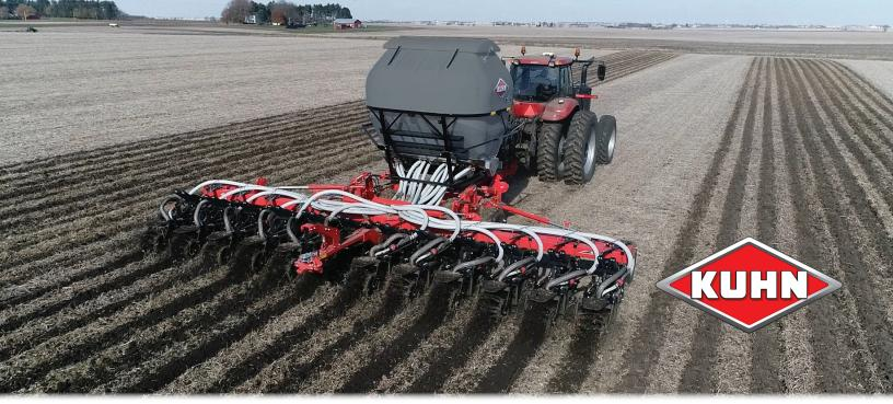
Strip-till allows precision tillage on 1/3 of the land while retaining all residue between the strips. This improves moisture infiltration into the strip and reduces rainfall runoff from the field, while providing a warm seedbed for early season planting. Residue between the strips helps retain moisture during dry times of the growing season while suppressing weed growth.
